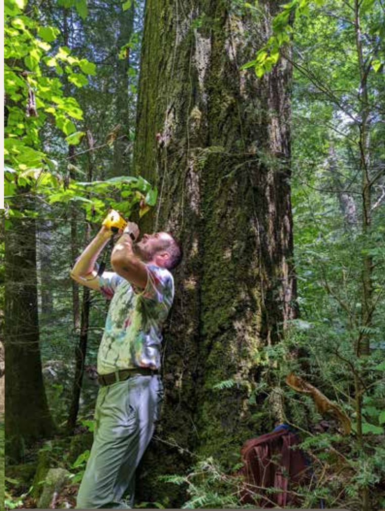
Figure 1 (above): Jimi Miller, former Tennessee Champion Tree Program (TCTP) intern, uses a hypsometer to measure a potential State Champion Tree.
